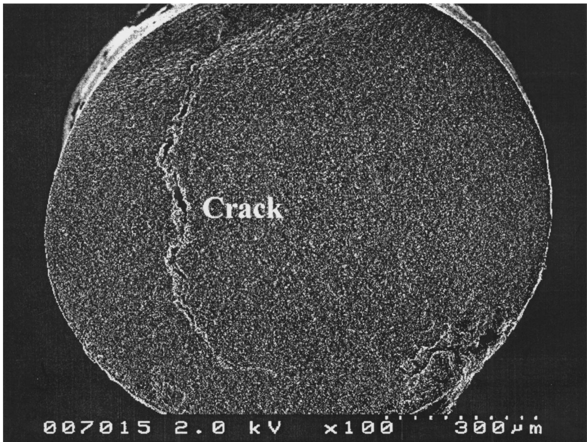
Figure 14 Fracture view of a SDK1 (2 h) 1 mm rod (sintered at 1600°C) showing a crack extended through the thickness.
